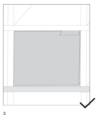
If after mounting, a side of the drawer rubs against the bottom element, the drawer will need to be adjusted.
