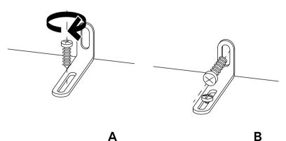
5 Align the bracket over the dowel and insert the supplied screw
